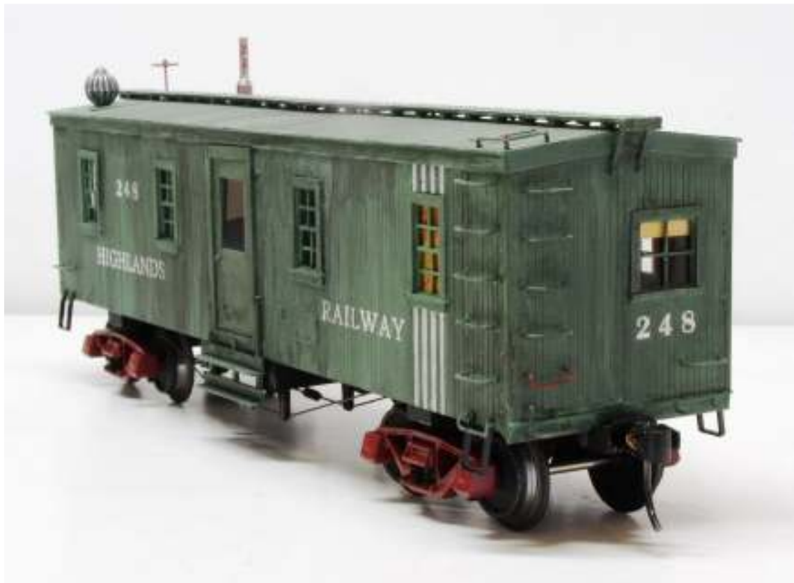
Completed car with freight trucks instead of caboose trucks as originally planned. I used both cans of green at the same time and let the colors blend. Glass added to windows. Decals were made for me by Rail Graphics. -JH
